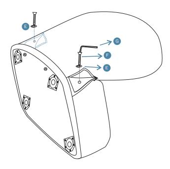
Peel back cushion cover as shown and attach to base and secure with  $2 \times 10^{-2}$  x screws (F) and  $2 \times 10^{-2}$  washers (E). Tighten with an Allen Key (G).
