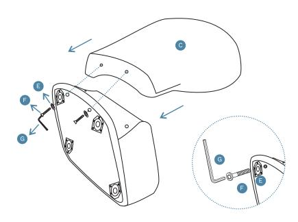
Attach 1 x cushion (C) to base as shown and secure with 2 x bolts (F) and 2 x washers (E). Tighten with an Allen Key (G).
